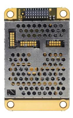
SATELLINE-M3-R4 is a flexible module which makes it a suitable unit for different uses. It is an updated version of M3-R3 module. It has two modulations more; 8FSK and 16FSK which gives more speed to the radio interface.
